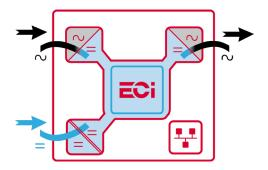
The modular inverter eliminates all single points of failure with full scalability; up to 32 modules in parallel and high efficiency of up to 96% in AC to AC conversion, and above 93.5% in DC/AC conversion, hence reducing operating costs.
